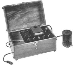
A portable rugged instrument for accurate reflectance measurements in
